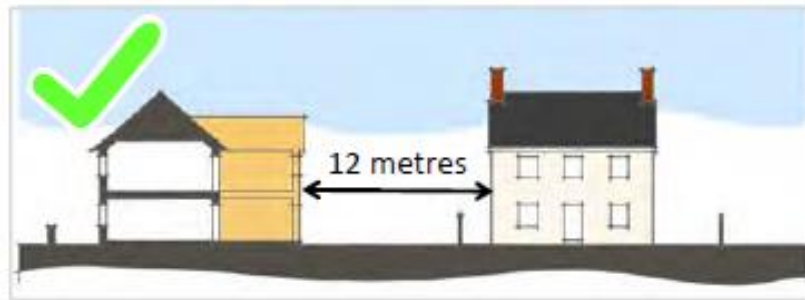
12m separation between an extension and wall with no windows
